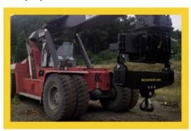
This Frame and this Beam transform any spreader into a Multipurpose transporter with a lower hook for General Cargo. Different configurations, lengths and SWL (Up to 80 Tons) according to customer's use and needs. Parking stand included.
