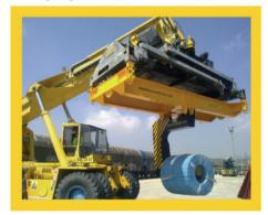
As an evolution from the BA-110 (check above these lines) the BA-110CP transform any Spreader for container into a Coilhandler. SWL and sizes are according to customer's use and needs.
