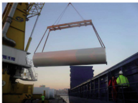
Frame BA-190 loading wind tower section
