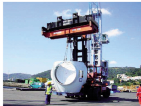
BA-110 for forklift handling wind rotor
